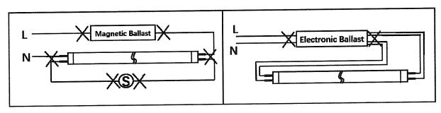
• Third Step: Install the LED tube and make the electrical connection
