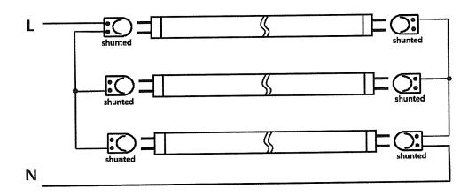
• Fourth Step: Affix the field applied label to the light fixture. Then install the tube. The tube is both ends wiring connection
